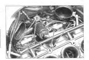
Stick Coil (Ignition Coil together with Spark Plug Cap) Installation
