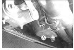
· Remove the muffler mounting nut [A].
