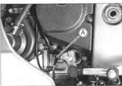
Pickup Coil Cover Oil Pressure Switch Terminal [A]
